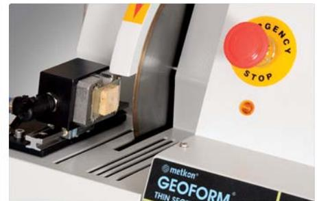
GEOFORM is a universal product that can be used for precision sectioning, re-sectioning and grinding operations
