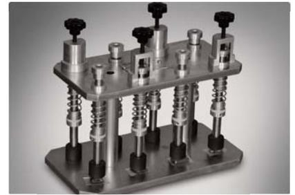
Fixture for mounting specimens to glass slides for thin-sectioning, provides a uniform thickness of bonding material between the specimen and the glass slide, spring activated loading system with capacity upto 8 specimens, easily plceable on hot plate
