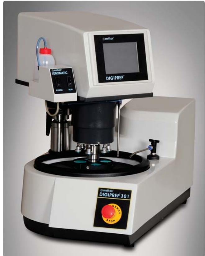
Upon completion of the cycle, an acoustic signal lets the operator know that the cycle is over and the samples are ready for the next step. When required, it is also possible to intervene in the program and change the parameters without stopping the instrument.
